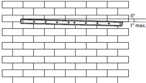
**CHECK WITH A SPIRIT LEVEL THAT THE INSTALLATION IS HORIZONTAL!**
