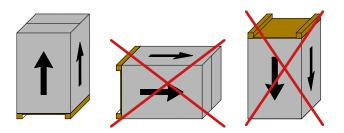
Handling with forklift truck: - Chiller on pallet
