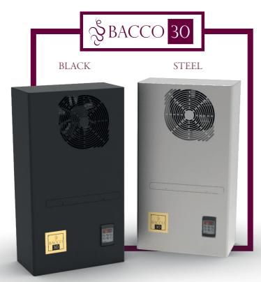
The structure of **BACCO 30** is made entirely of **AISI 304 stainless steel**, brushed on the outside or painted in anthracite colour. It contains the low noise rotary type compressor, the cooling coil, and the 1Kw electric heater for the production of hot air.
