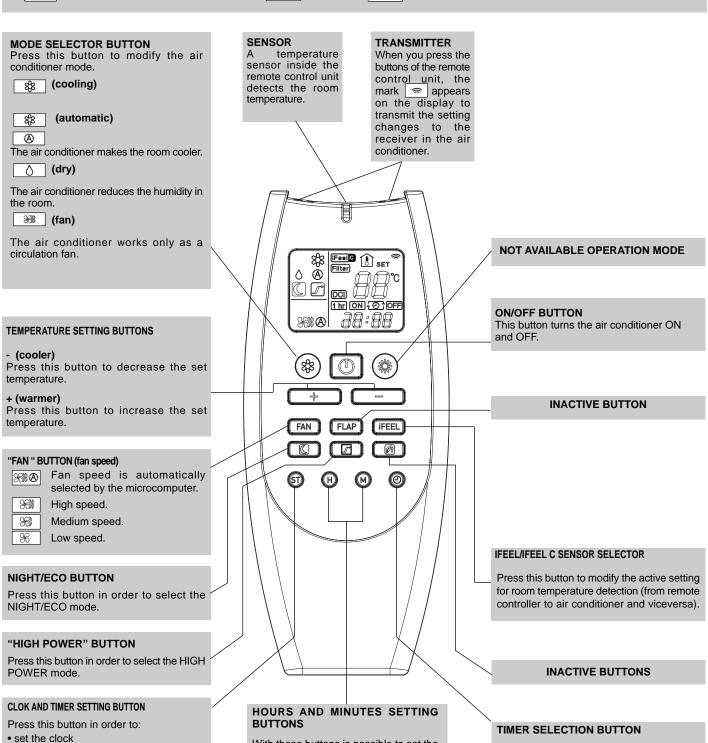
With these buttons is possible to set the clock and the timer. For details refer to paragraphs "SETTING THE HOUR" and 'SEŤTING THE TIMER".
