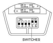
Insert two AAA alkaline batteries of 1,5 V-DC making sure that point in the direction marked in the battery compartment. The displayed time flashes.
